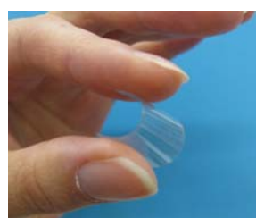
▲ Fig.1: Photograph of a transparent conductive sheet made from a plastic material
