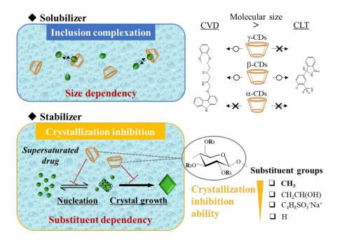
**Title:** The mechanism underlying the stabilization of supersaturated drugs with cyclodextrins. **Caption:** Schematic illustration of inclusion complexation and crystallization inhibition abilities of cyclodextrins
